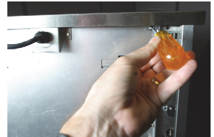
Figure 2: The top is secured with tabs, which extend down and are captured by screws just under the lid.
